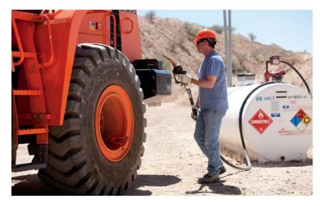
chemical structures and lead to pump, filter and injector problems. All machine fluids should be handled in a dedicated fluid containment area and stored in a manner that maintains a maximum level of cleanliness.
